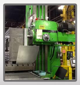
Our 5" Ceruti Bar, offers our customers, cost-effective machining, for their large precision fabrication needs. The rotary table of our horizontal boring bar allows multi-axis machining of complex and contoured parts without repositioning. The rotary table indexing allows three dimensional precision machining of our customers fabrications.
